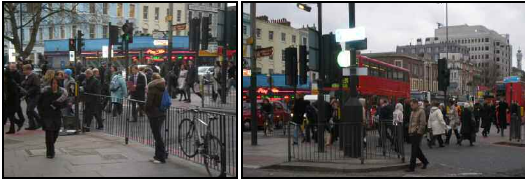
Plate 4.18: Insufficient crossing capacity across York Way (C9/C10)
