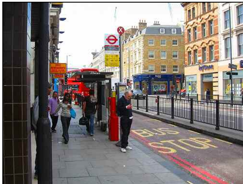
Plate 4.27 Narrow waiting area capacity at PT5 with barriers causing deviations
