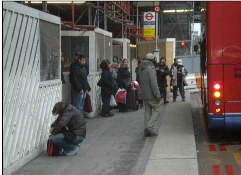
Plate 4.25 Narrow footway width causes conflict between waiting pedestrians and passing flows at PT7
