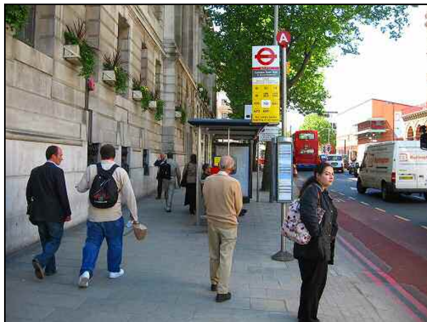
Plate 4.29 Bus shelter causes a pinch point at PT6 which can create user conflict during peak hours
